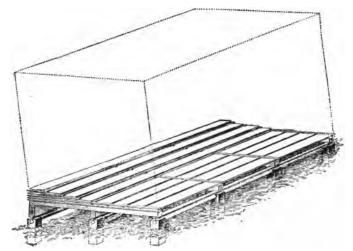
Fig. 80.—Lumber piled sidewise on cement and metal foundations.
